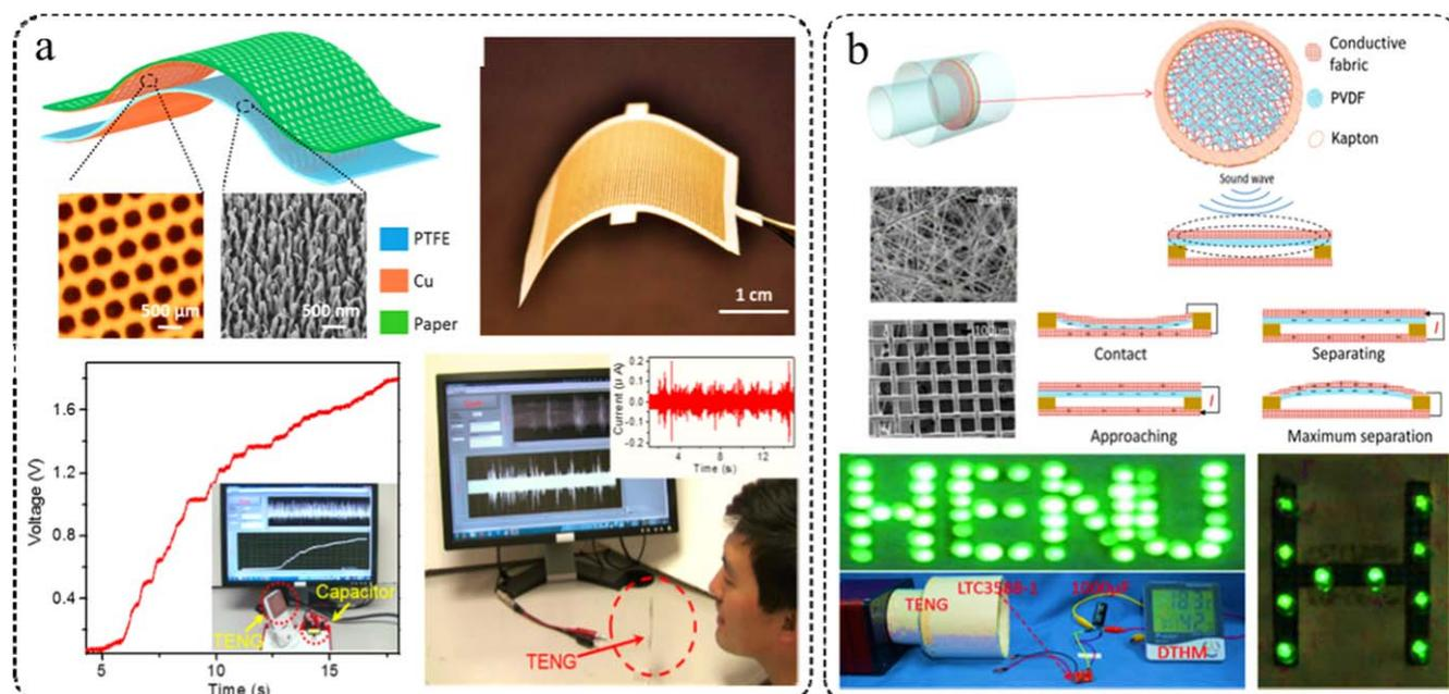
**Figure 11.** Thin-film TENGs used to collect sound energy. (a) Schematic and photograph of an as-fabricated paper-based TENG. (Reproduced with permission from [30]. Copyright 2015 American Chemical Society). (b) Structural design and working principle of the SD-TENG. (Reproduced with permission from [31]. Copyright 2019 Elsevier Ltd).
