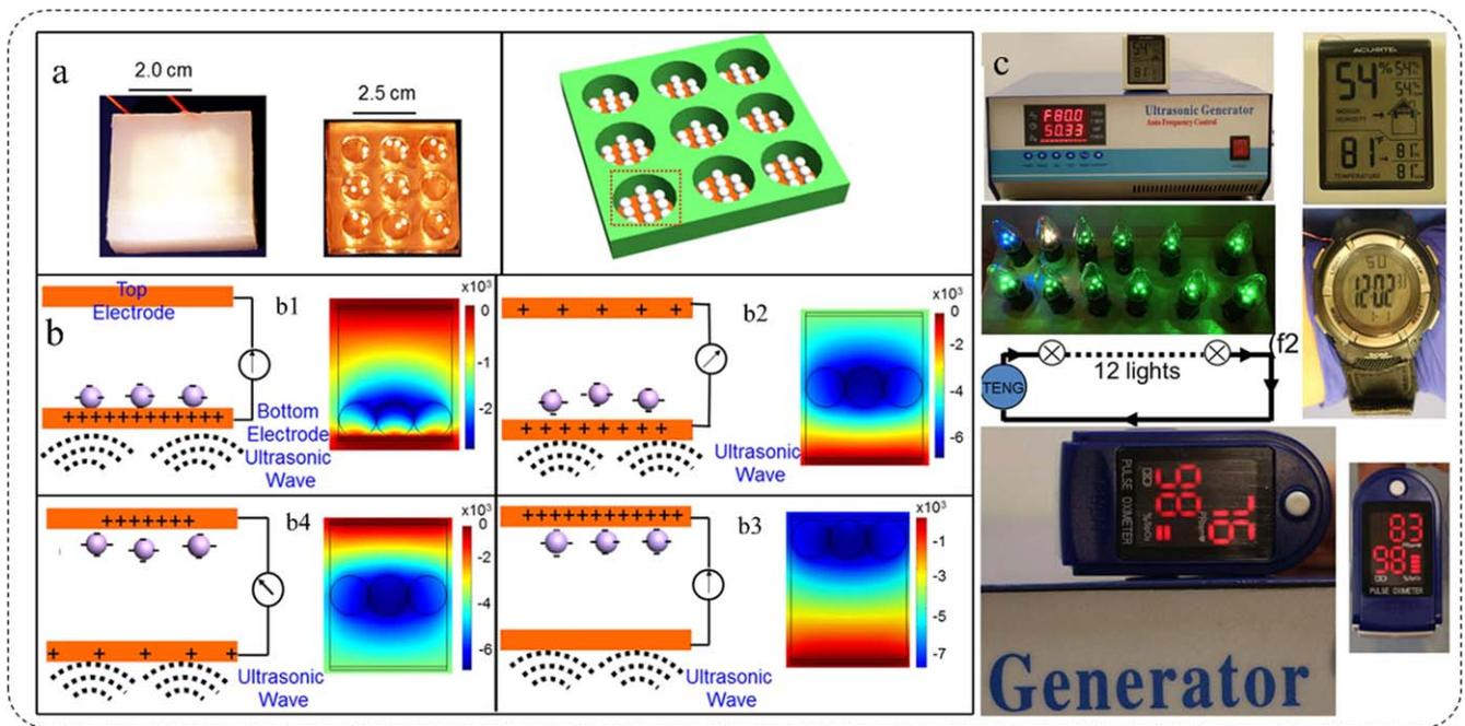
**Figure 13.** Design, working principle, and application of the acoustic energy TENG. (Reproduced with permission from [125]. Copyright 2017 Elsevier Ltd). (a) Photograph showing the packaged TENG and inter-structure of the TENG. (b) Working principle of the device and finite-element simulation. (c) Photographs of the digital temperature-humidity weather monitor and the electrical watch continuously driven by the TENG.
